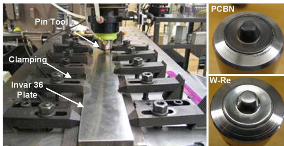
Fig. 2 Friction stir welding setup showing Invar plate, clamping, and pin tools
