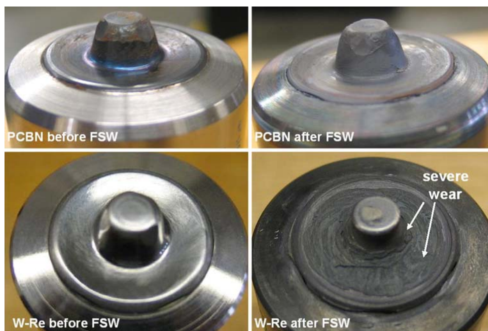
Fig. 6 Appearance of PCBN and W-Re pin tools before and after friction stir welding of Invar
